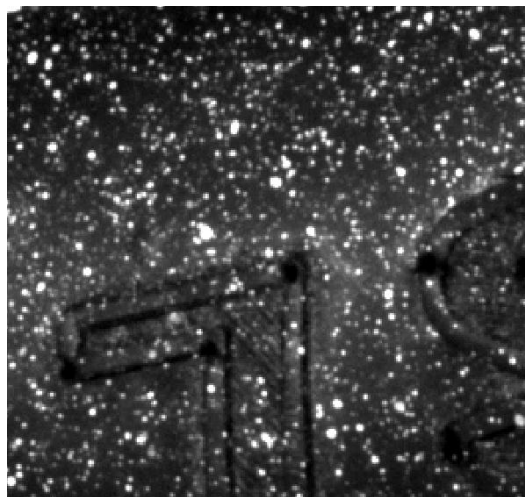
FIGURE 15: HIGH-CONTRAST, RANDOMIZED SPECKLE PATTERN APPLIED TO TIRE SURFACE
