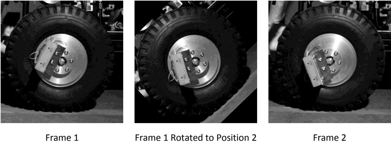
FIGURE 45: EXAMPLE OF RE-ROTATION APPLIED TO TIRE IMAGES
