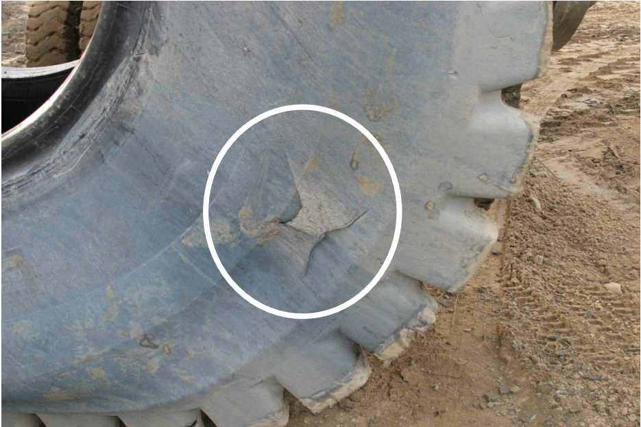
FIGURE 4: SIDEWALL CUT IN HAULAGE TIRE
