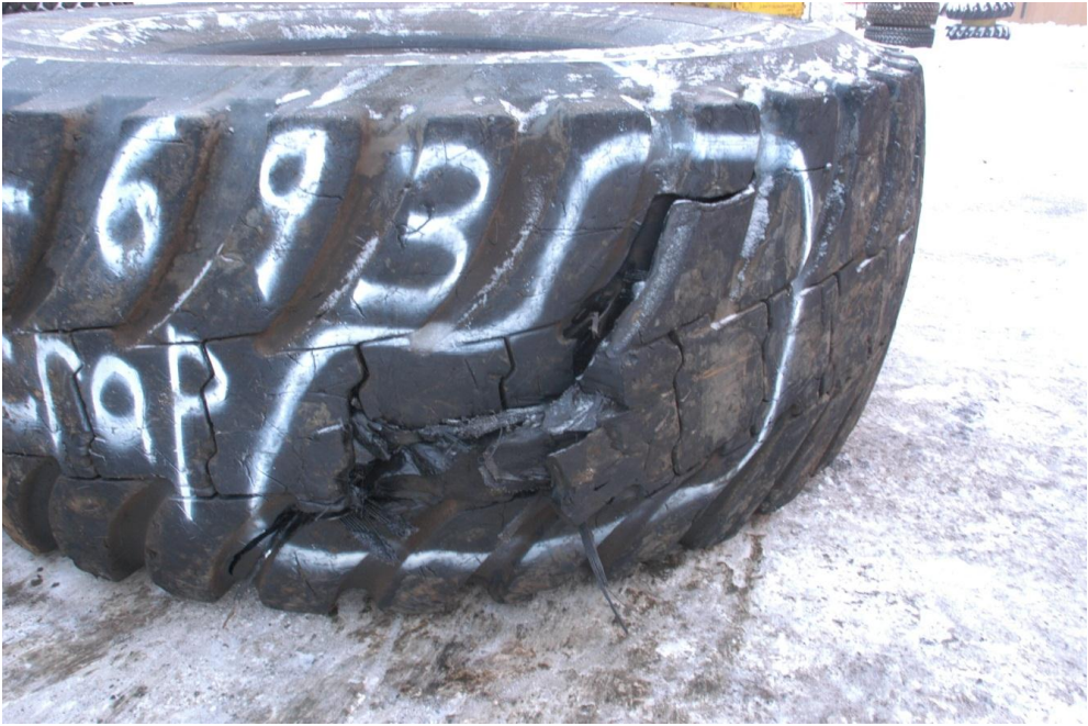
FIGURE 3: HAULAGE TIRE WITH TREAD CUT AND SEPARATION
