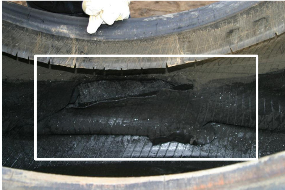
FIGURE 5: INTERNAL VIEW OF BELT SEPARATION IN HAULAGE TIRE
