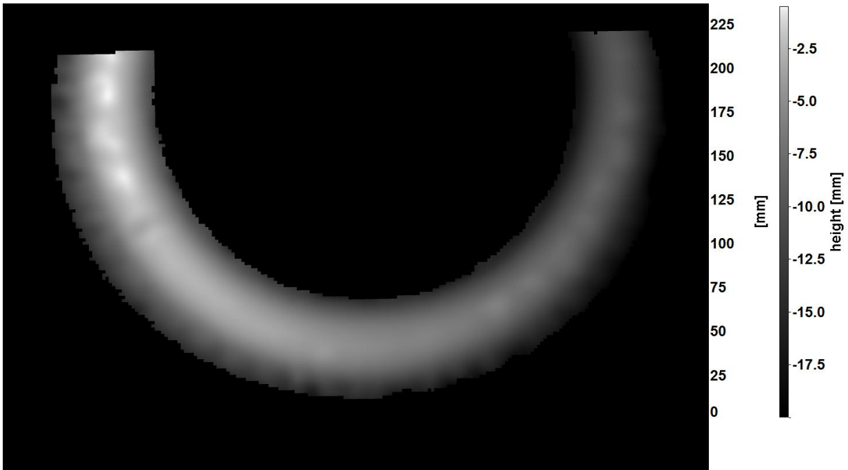
FIGURE 39: SOFTWARE RECONSTRUCTION OF 3D TIRE SURFACE
